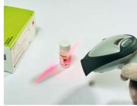
The external barcode reader identifies material and checks the lot number and expiration date.
